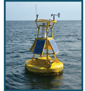
Buoys with sensors that monitor ocean chemistry provide critical data for studying acidification.
