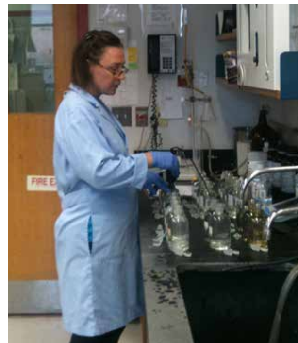
At the IEC District Laboratory on Staten Island, N.Y., NEIWPCC's Inna Golberg tests water samples for biochemical oxygen demand, a key indicator of water quality.
