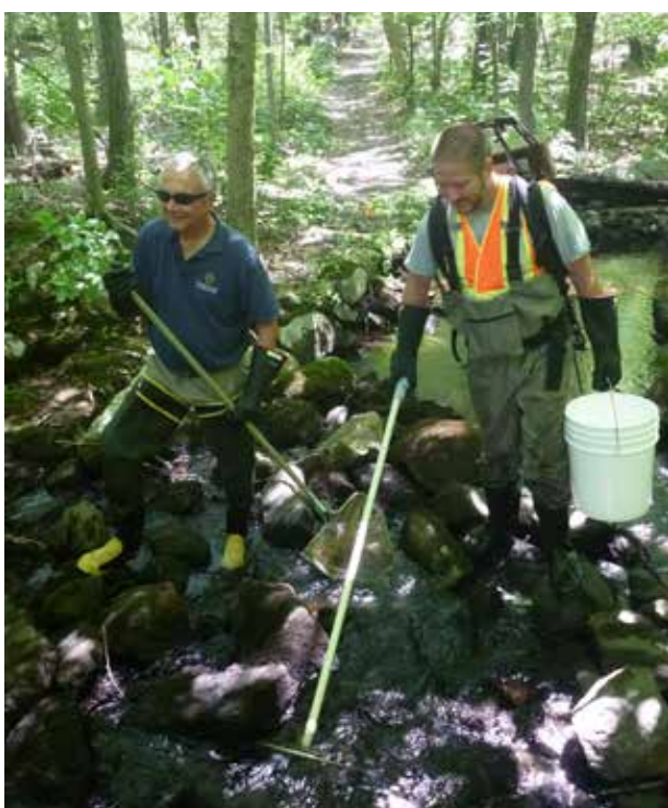
At left: During a visit to Rhode Island's West River to collect fish community data, Alan Libby (left) of RIDEM's Department of Fish and Wildlife and NEIWPC's Mark Nimiroski employ the technique known as electrofishing. Electricity is used to temporarily stun fish so researchers can easily capture and study the fish before returning them unharmed to the water. Above: A collection of photos of some of the catch during the river assessments. Clockwise from lower left: a bucket of fish caught during electrofishing, pumpkinseed sunfish, American eel, juvenile brook trout.
